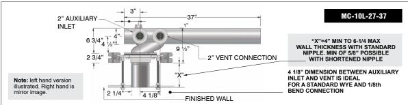
Note: 10 1/2" (267) minimum space required between front of foot and rear of anchor support. 8" (203) minimum in wall space required between back of rear anchor support and back of in wall foot supports.
