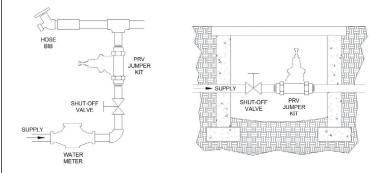
NOTE: THE BODY MUST ALWAYS BE USED WITH THE GASKETS FOR THE PRV TO FIT THE SPACE WHEN THE JUMPER KIT IS REMOVED.
