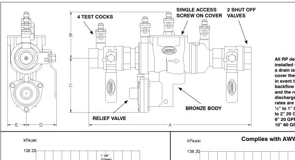
All RP devices must be installed where a drain is available to cover the discharge in event there is a backflow condition and the relief valve discharges. Discharge rates are as follows: 1/2" to 1" 5 GPM, 1 1/4" to 2" 20 GPM, 2 1/2" to 6" 20 GPM, and 8" to 10" 60 GPM.
