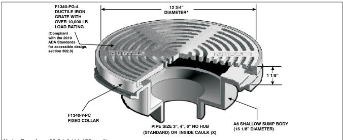
Note: Free Area 68.9 in<sup>2</sup> (44,452 mm<sup>2</sup>) F1340-Y-Q Series meets ANSI/ASME floor drain standard A112.6.3-2001
