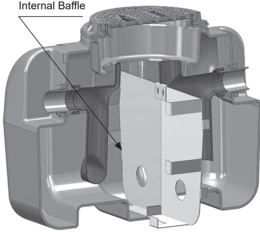
BIG-750-IB - with internal baffle
