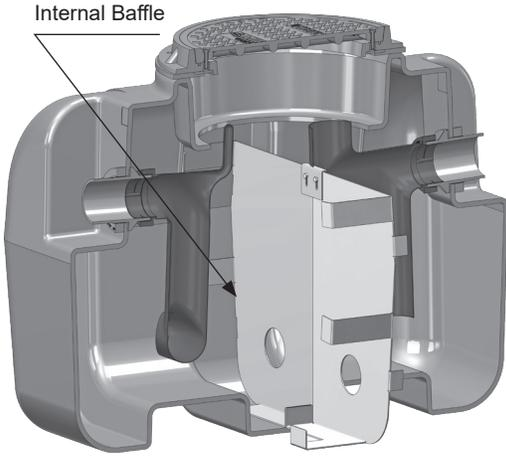
BIG-750-IB - with internal baffle
