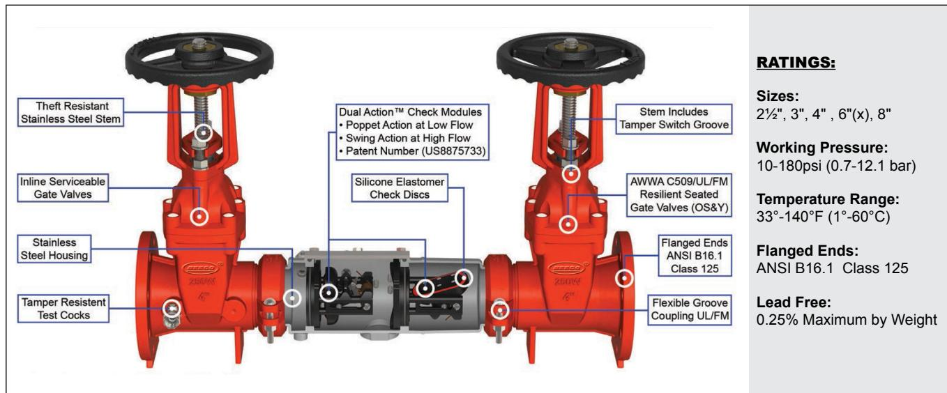
**Features:** Single access cover for fast service. Swing away clamp for ease of removing checks. Modular design reducing number of spare parts. Self contained check so there is no pressure to relieve when changing the seats.
