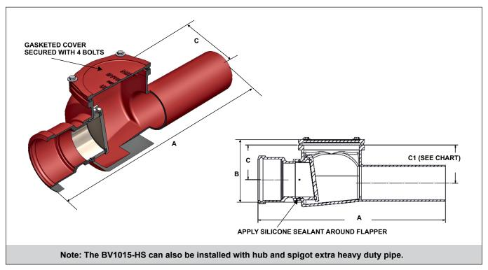
**Note:** Do not use for pressurized applications; for gravity flow only. Backflow protection is prevented when the valve is obstructed by debris or sludge; clean regularly.
