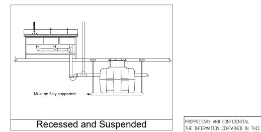
**MIFAB** 75GPM HDPE GREASE BIG-750 SCALE: 1:11 WEIGHT SHEET 1 OF 1
