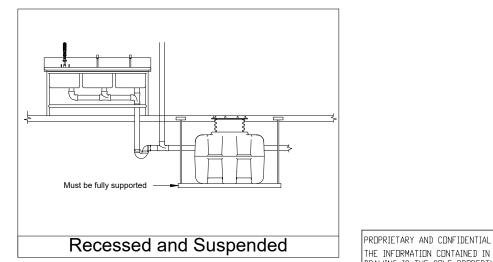
**▲ MIFAB** 50GPM HDPE GREASE INTERCEPTOR REV SIZE |DWG, ND, SHEET 1 DF 1
