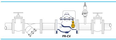
The Model PR-CV reduces high pressure from near zero to the maximum flow rate without the need for an additional Low-Flow Bypass. If the system is subjected to potentially static downstream conditions, a Pressure Relief Valve (½" or larger) is recommended for additional system protection.
