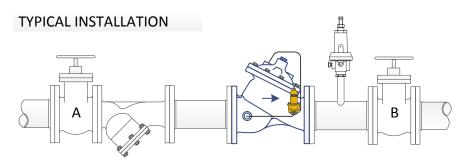
The Model HF5PR reduces high pressure from near zero to the maximum flow rate without the need for an additional Low-Flow Bypass. If the system is subjected to potentially static downstream conditions, a Pressure Relief Valve (½" or larger) is recommended for additional system protection.
