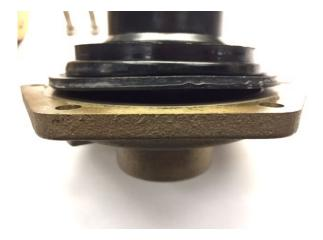
3) Line up the piston assembly so that the diaphragm is against the cover without pushing the piston in such that the diaphragm is not distorted. Install the cover assembly screw in to hold the piston assembly in this condition while putting the body and cover together. Note that the drawing shows the approximate range to set the screw for setting the piston assembly.
