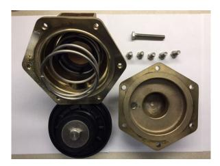
2) Place the piston assembly into the cover after applying the proper grease to the piston o-ring.
