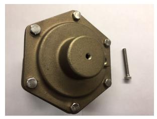
6) Finally, test the valve and make sure it opens at a pressure differential between 2.5psi and 3.5psi.
