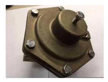
5) Unscrew the cover assembly screw and remove it from the assembly. The valve should function properly now.
