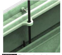
STEP 8 Tighten the zip ties around the pins of the interceptor or through the next hole if using more than one extension
