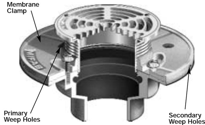
choose from literally thousands of products from many manufacturers. A mechanical designer has to be careful at every turn to make sure he has decided between non tilt or tractor grates, between ductile and gray cast iron, between adjustable and non-adjustable top assemblies, heel proof or non heel proof grates. In short a baffling array of options that do little to improve the basics of the design, i.e. free area and load bearing characteristics.
