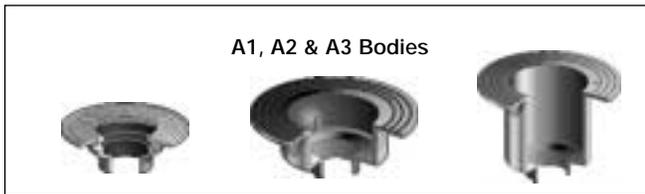
rates. The shallow design of the A1 body allows for installation in slabs of minimum thickness. **Because a membrane clamp is usually not required (the majority of drains and cleanouts are installed slab on grade), MIFAB's A1 body design incorporates an integral female thread (4" N.P.S.) to receive adjustable strainers or cleanout tops.**
