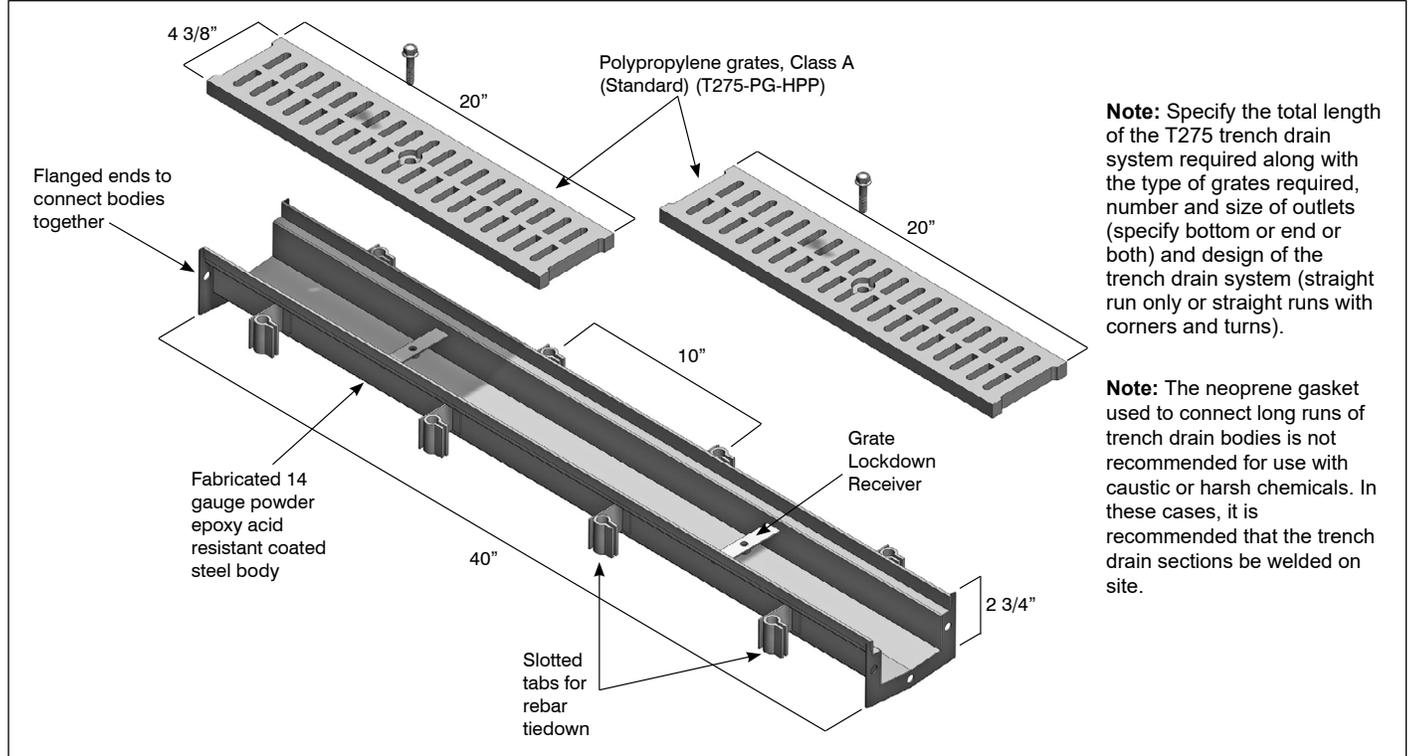
**Note:** Specify the total length of the T275 trench drain system required along with the type of grates required, number and size of outlets (specify bottom or end or both) and design of the trench drain system (straight run only or straight runs with corners and turns).
