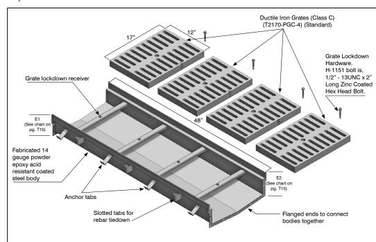
Note: The neoprene gasket used to connect long runs of trench drain bodies is not recommended for use with caustic or harsh chemicals. In these cases, it is recommended that the trench drain sections be welded on site.
