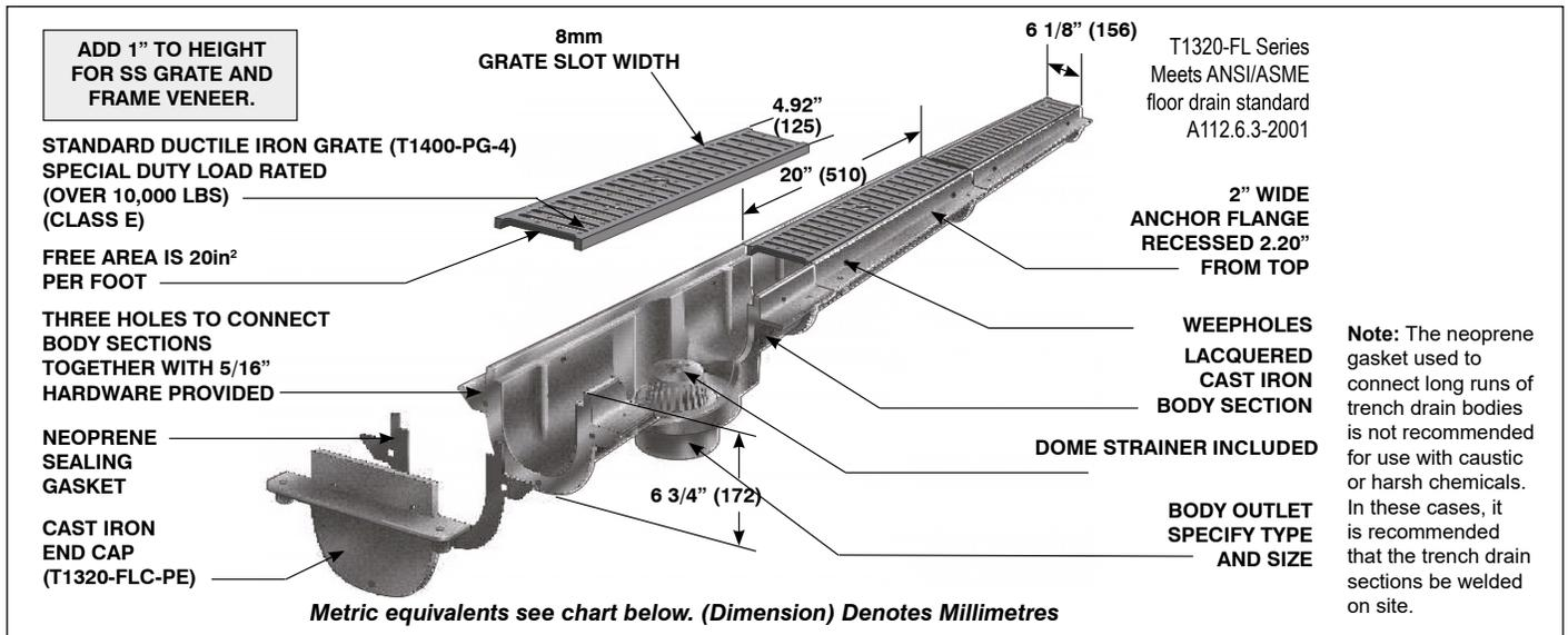
**Note:** Specify total length of trench drain required in 20" long sections. Section "A" is standard with a bottom outlet (specify bottom outlet connection type and number and location of outlets required). Section "B" does not have a bottom outlet. Any number of Sections "A" and "B" can be bolted together to produce any length required.
