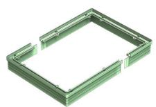
STEP 3 Apply silicone sealant in the groove between each body component push them together
