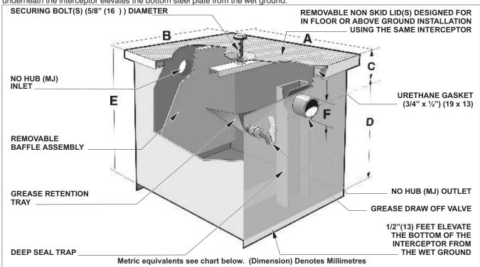
**Note:** The "C" dimension detailed above is from either the middle of the inlet or the outlet to the top the interceptor. The inlet and outlet dimensions are always the same.
