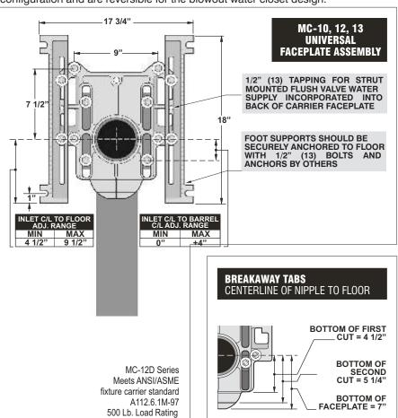
**Note:** 8" tapered thread ABS nipple shipped standard with MC-12D Series carriers. The universal faceplate assembly accepts all nipple variations, rolling thread (-OR), cast iron (-CI) and tapered thread ABS with adjustable horn (-AH).
