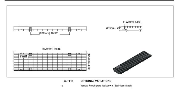
Load Class C- Heavy Duty, DIN 19580, 56,000 lbs. 1.162 psi. For commercial pneumatic tire traffic patterns and tractor trailers.
