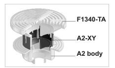
The A2-XY is used with A2 and A3 bodies to receive the F1340-TA, F1360-TA, F1440-TA and F1460-TA top assemblies. It has an adjustment range of 3 7/8" to 5 3/8". The top assembly can be adjusted side to side to align with the floor tiles without changing vertical height. This is a benefit in promenade areas where the installer must align square tiles with the drain top assembly. The A2-XY is independent of the body and the top assembly is independent of the A2-XY.
