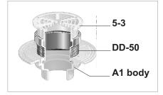
The DD-50 extension is used with A1 and A4 bodies to receive any strainer or cleanout top with a 4" N.P.S. shank. The DD-50 has an adjustment range of 1 1/2" to 2 5/8".
