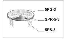
The SPR-5-3(-1 for NB) is used with 5-1 and 5-3 strainers to increase the height of the strainer to match discrepancies in the finished floor grade. Any number of rings can be added on top of each other. Each ring adds 3/8"of height. Simply remove the grate, place the SPR-5-3(-1 for NB) into the cast in place shank, and then screw the grate into the ring. Longer bolts are provided by MIFAB. The vertical height of the strainer can be adjusted after the drain is poured in place.
