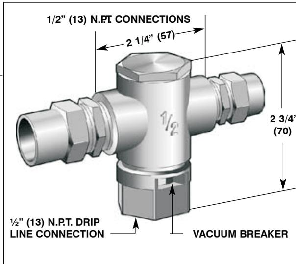
**Specification:** MIFAB® S series MI-TSP-3-NPB brass trap seal primer with removable poppet, integral vacuum breaker, gasketed access cover, ½" (13) N.P.T. inlet and outlet connections, complete with ½" (13) sweat connection adapters and ½" (13) N.P.T. drip line connection.
