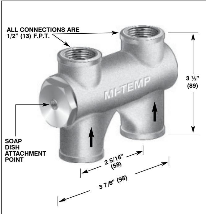
**SPECIFICATION:** MIFAB Series MI-TEMP-NPB automatic pressure balance valve complete with rough chrome plated cast brass body, type 304 stainless steel piston and shell and two 1/2" (13) F.P.T. inlet and two 1/2" (13) F.P.T. outlet connections. Unit complete with brass plug at end tapped 1/8" (3) for soap dish attachment. Product complies with the AB 1953 low lead requirements.
