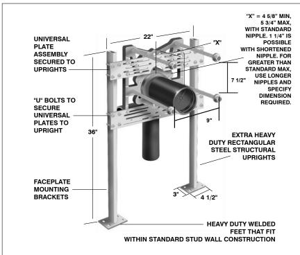
MC-62 Series Meets ANSI/ASME fixture carrier standard A112.6.1M-97
