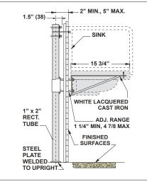
MC-34 Series Meets ANSI/ASME fixture carrier standard A112.6.1M-97
