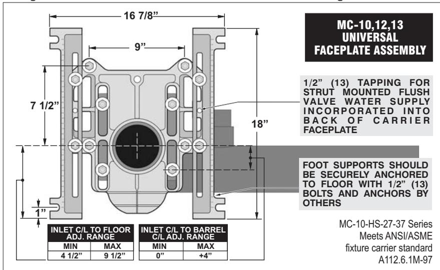
**Note:** 8" tapered thread ABS nipple shipped standard with MC-10 Series carriers. The universal faceplate assembly accepts all nipple variations, rolling thread (-OR), cast iron (-CI) and tapered thread ABS with adjustable horn (-AH).
