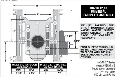
Note: 8" tapered thread ABS nipple shipped standard with MC-10 Series carriers. The universal faceplate assembly accepts all nipple variations, rolling thread (-OR), cast iron (-CI) and tapered thread ABS with adjustable horn (-AH).
