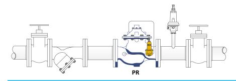
The Model PR reduces high pressure from near zero to the maximum flow rate without the need for an additional Low-Flow Bypass. If the system is subjected to potentially static downstream conditions, a Pressure Relief Valve (½" or larger) is recommended for additional system protection.
